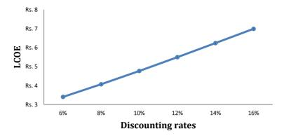
Figure 4c LCOE of FBR as a function of discounting rates
