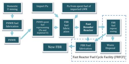
**Figure 1** Fuel cycle for Fast Breeder Reactor using reprocessed spent fuel from PHWRs including possibility of reprocessing LWR spent fuel and importing Pu.
